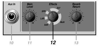
The PA4FX features Crate's On-Board *Digital Signal Processing* (**DSP**) technology that was designed specifically for use with instruments and vocals. This provides a large selection of digital reverbs, effects and delays. Select the type of effect desired by rotating the Effects control (#12). This control is divided into five sections: Small Area Reverbs (**SAR**), Large Area Reverbs (**LAR**), Special Reverbs (**SPR**), Delays (**DLY**) and Multiple Effects (**Multi**).
