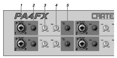
**1. BAL. INPUT:** Connection to the mixer is made here by means of a balanced 1/4" high-Z or XLR-type low-Z plug. The wiring for this combination jack is as follows: 1/4" Tip = signal +, Ring = signal –, Sleeve = signal ground; XLR pin 1=signal ground, pin 2=signal +, pin 3=signal –.
