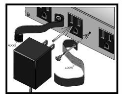
1: Cut apart a hook-and-loop strap where the two parts join in the middle.
