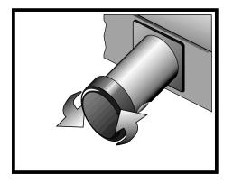
1: To Avoid the risk of electric shock, turn the lights off (dimmer control fully counter-clockwise) or disconnect the unit's power cord from its power source. Pull the light tube out from the unit.
