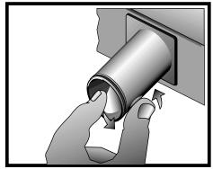
**3:** Using your thumb and forefinger, gently rotate the bulb counterclockwise. Use your thumb to work the bulb through the hole along the bottom of the light tube while pressing down on the bulb with your finger.
