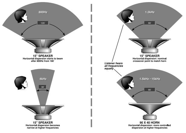
This chart illustrates different diameter cone loudspeakers and their typical dispersion characteristics:
