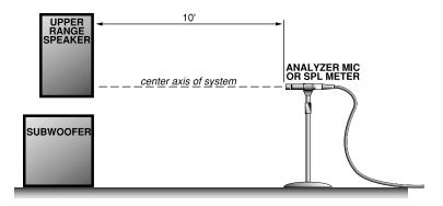
Of course, this will only get the two speakers close to an electrical balance and more equalization will be required to achieve the best sound and balance.
